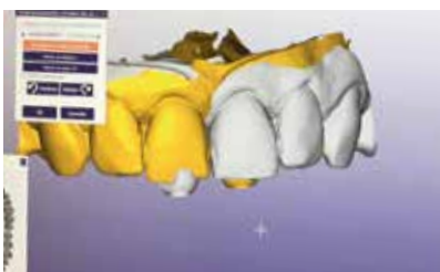
Prosthesis modeling, file is handed over to milling center.
